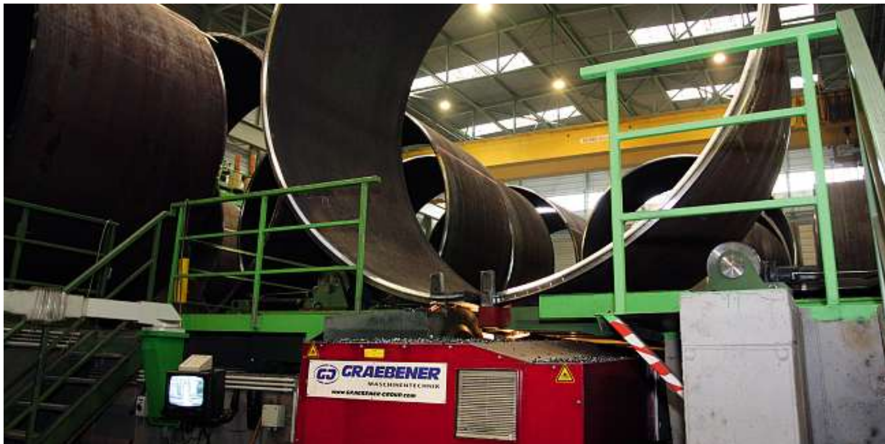
Especially the long (photo) and the circ seam milling machines have become integral working stations of a wind tower production.
