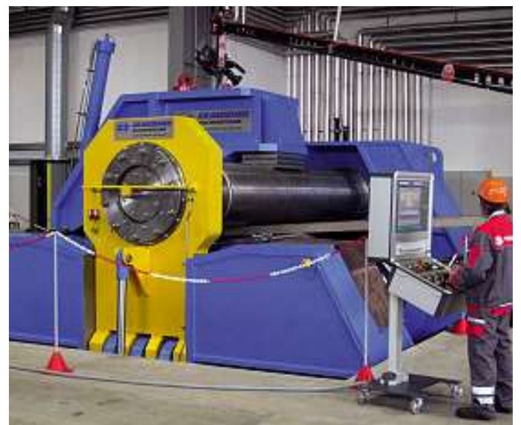
The compact design of the machine is even more illustrated when most of the machine is embedded in the foundation.
