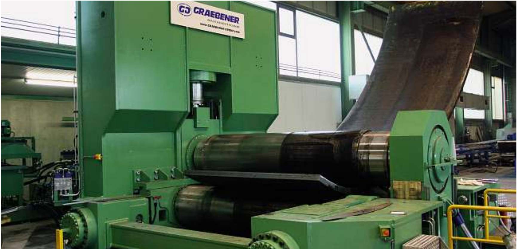
The 3-roll bending machine is a multi-talent – for the bending of pipes and shells, vessels, apparatuses and even cones.
