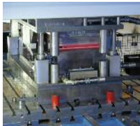
Dies open and closed, stationed in an AP&T hot-stamping line. The closed die performs forming and cooling functions.
